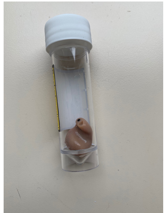
Figure 2 In-the-ear hearing aid retrieved with button battery inside.
