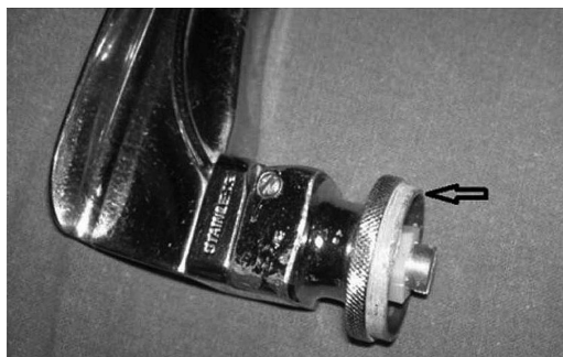
Figure 2 Failed welding at hinge piece.
