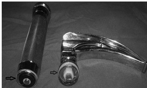
Figure 1 Hinge piece separated from knurled barrel of handle.
