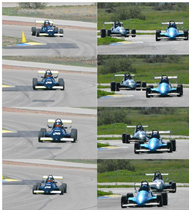
**Figure 1** Driver's head position in sequential images taken on entry, mid-corner and corner exit without the halo-type structure (left-hand sequence) and with the halo-type structure (right-hand sequence). An increase in right lateral flexion can be seen particularly on corner entry and corner exit.
